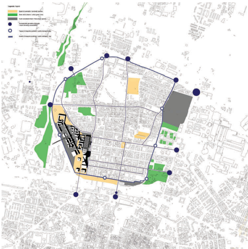
FIGURE 19.3 The structure of the “Bolognina” centrality field, highlighting the annular mobility layout with respect to which the new metropolitan-type urban centrality project is established (scale 1:5000).
