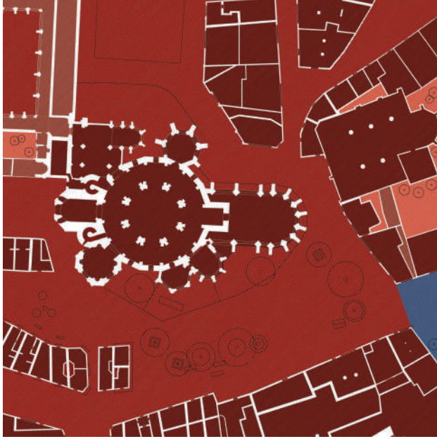
FIGURE 4.3 Red-blue plan of the Aachen cathedral and surroundings, original scale 1:666, drawn by students of the class Grundlagen des Entwerfens – Stadtraumgestaltungen, Kartierung städtischer Räume in 2019.
