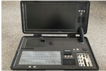
Figure 18. Autonomous underwater vehicle operating system.
