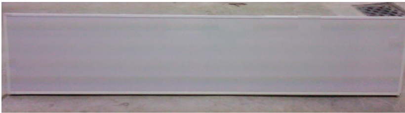
Figure 5. Rigid member (PVC): length 1.9 m; density 181.05 (kg/m 3 ); weight 8.6 kg, thickness 0.02 m.
