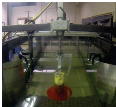
Figure 4. Photo showing the Marine Ocean and Offshore Research (MOOR) wave tank with the model and actuator in the foreground. Wave deflectors on either side for still water runs.
