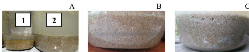
Figure 2. Desert sand leaching (A, 1 - abiotic control, 2 - bioleaching) and details desert sand color after 1 day of bioleaching (B) and after 1 months of bioleaching (C).
