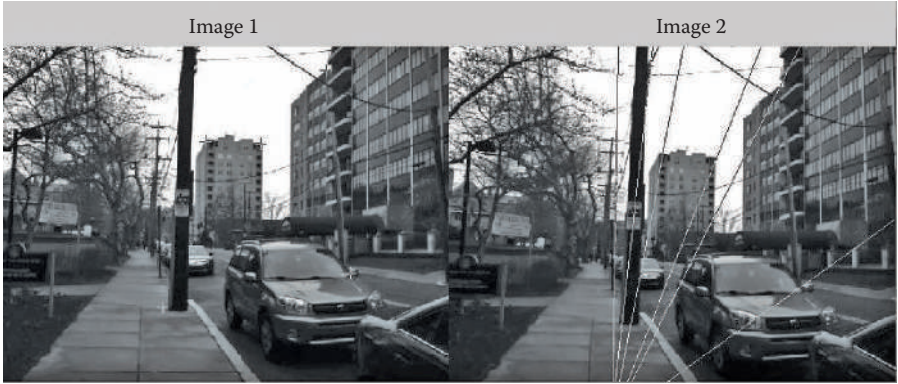
FIGURE 9.13 Feature points in Image 1 versus Epipolar lines in Image 2.
