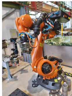
Figure 1. Kuka KR120 with gripper, used to executed planned paths in a series of criteria-validating experiments.
