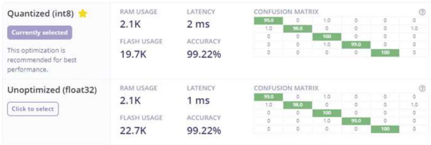
Figure 12.7 A comparison between int8 quantized and unoptimized versions of the same model, showing the difference in performance and results.
