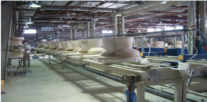
Figure 3.2 Ceramic sanitaryware casting industrial assembly. (Source: Fortuna, A., Fortuna, D. M., and Martini, E. (2017) An industrial approach to ceramics: sanitaryware. Plinius , 43, 138–145).
