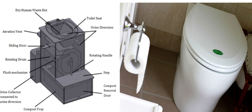
Figure 3.4 Schematic of a composting toilet with urine diversion (Source: Wikipedia contributors, 31 December 2020).
