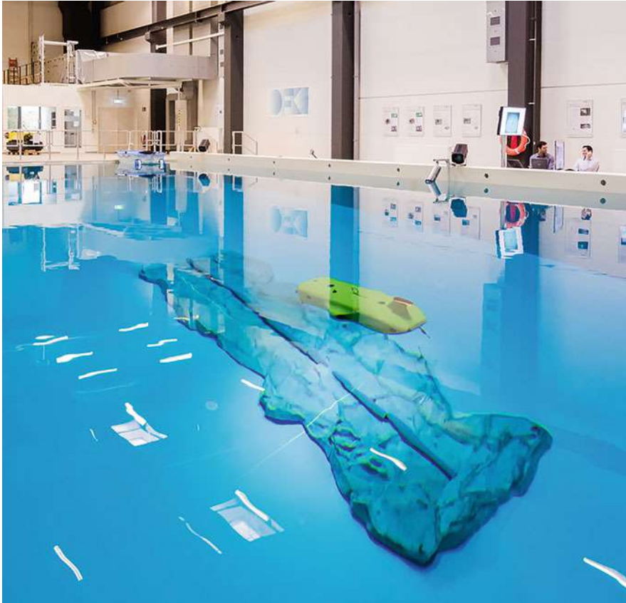
Fig. 4.4 Mission scenario of a pipeline inspection mission (Source: DFKI GmbH, Jan Albiez)
