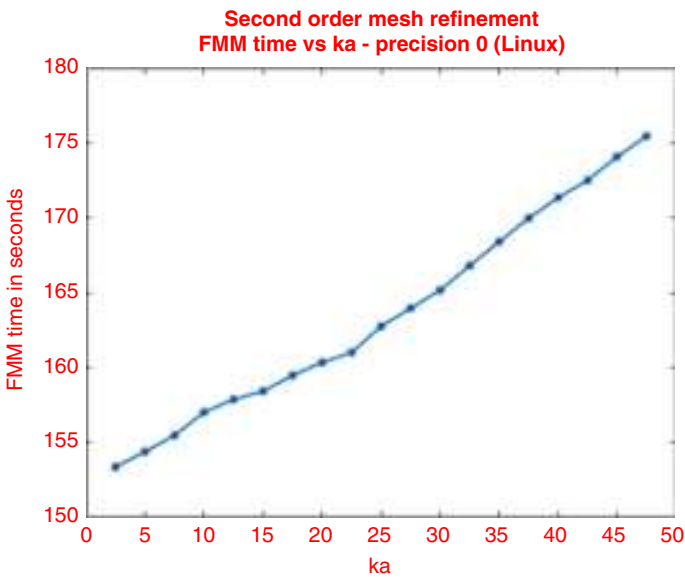
Fig. 34 Average FMM runtime for the doubly refined models in MATLAB on Linux is plotted with respect to values of ka . The demanded precision is two digits accuracy
