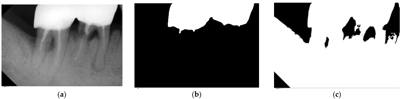
Figure 5. The result of the preprocessing. (a) Original image. (b) Directly binarized image. (c) Adjusted grayscale image.
