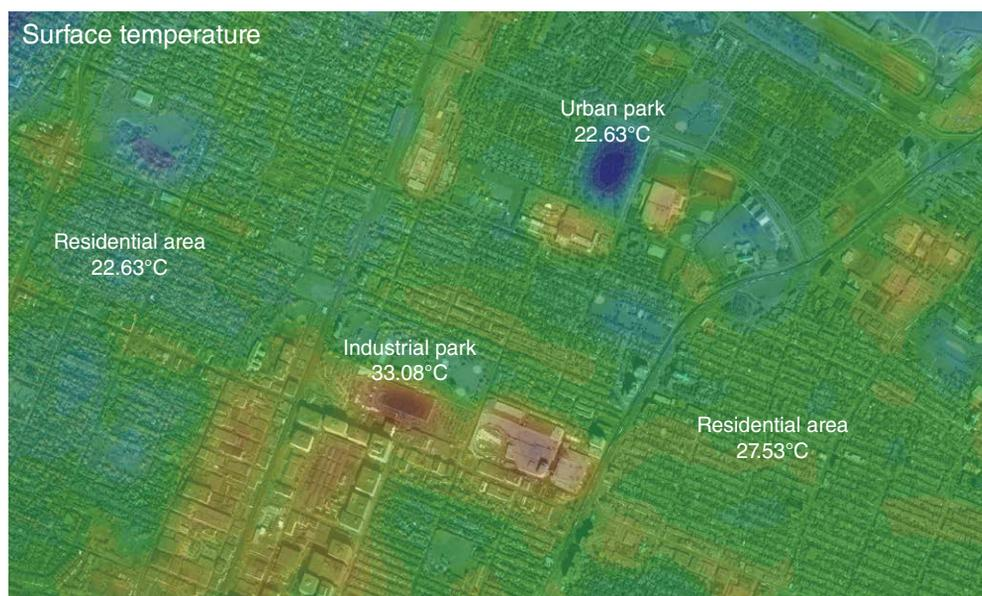
**Fig. 2.3.2.** Example of Landsat-8 Thermal Infrared Sensor (TIRS) thermal band measurements, dated 20 August 2013, superimposed on detailed satellite imagery of an urban area in Montreal, QC, showing the close relationship of land use categories and thermal conditions. Surface heat islands are depicted in red; cooler areas are represented in shades of green and blue. (From: Philippe Martin, ECCC.)
