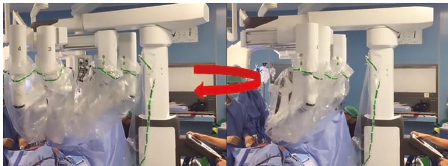
**Fig. 15.2** The boom system can be re-orientated to every part of the patient by undocking the port performing a re-targeting and a new docking phase
