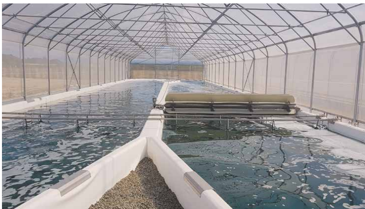
Figure 2. Spirulina production in raceway pond in a greenhouse (Grosseto, Italy; Source: Algen archive).
