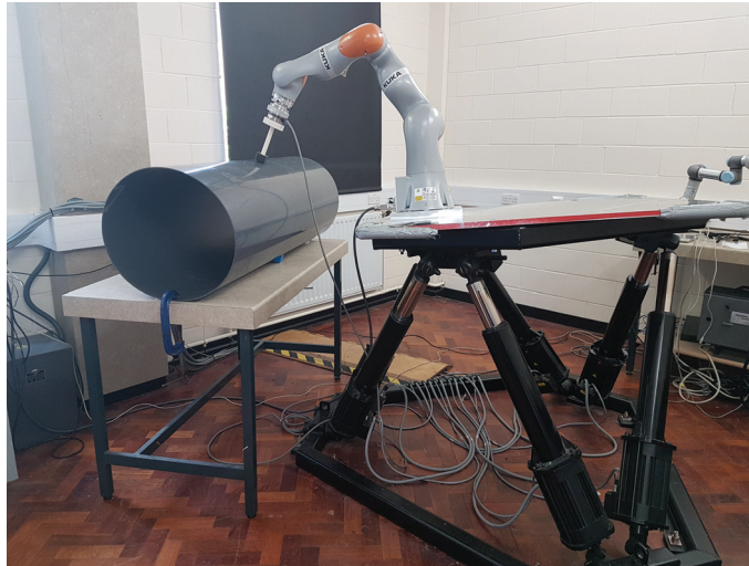
Figure 3. Simulating the UVMS with a real KUKA IIWA14 robot manipulator fixed on the Stewart parallel manipulator platform interacting with a pipe.
