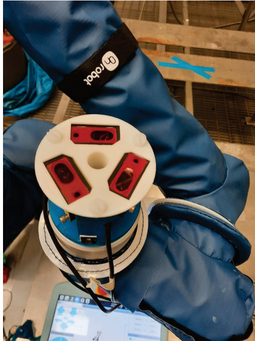
Figure 11. The tri-laser holder, attached to the UR10e flange. The design with rotational symmetry around axis 6 of the robot minimised the footprint of the tool.
