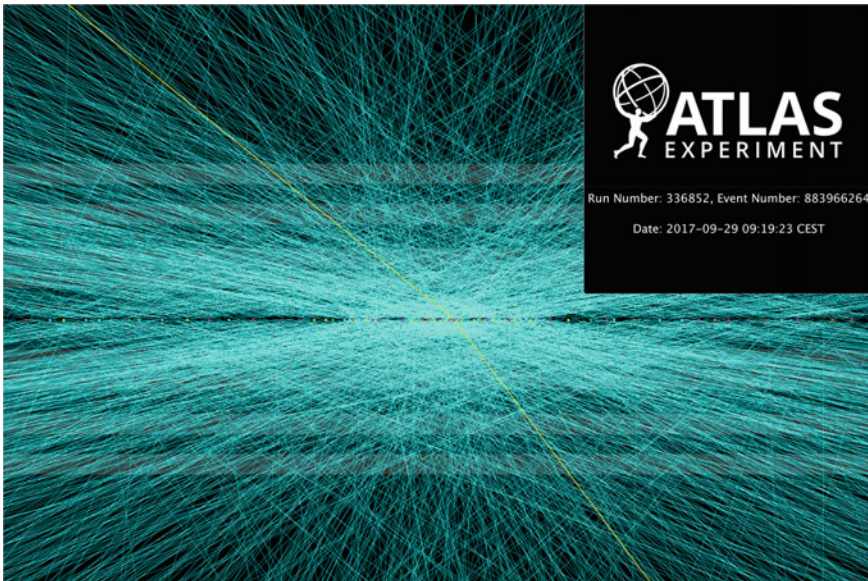
Fig. 6.3 Event display obtained from the real data in the ATLAS experiment. Reprinted under the Terms of Use from [3] ATLAS Experiment © 2022 CERN. All rights reserved. The reconstructed tracks are shown in the lines, and the vertex by the circles. There are 65 proton-proton interaction points on top of the one where Z boson is produced and decayed into dimuon. This dimuon is shown in yellow lines
