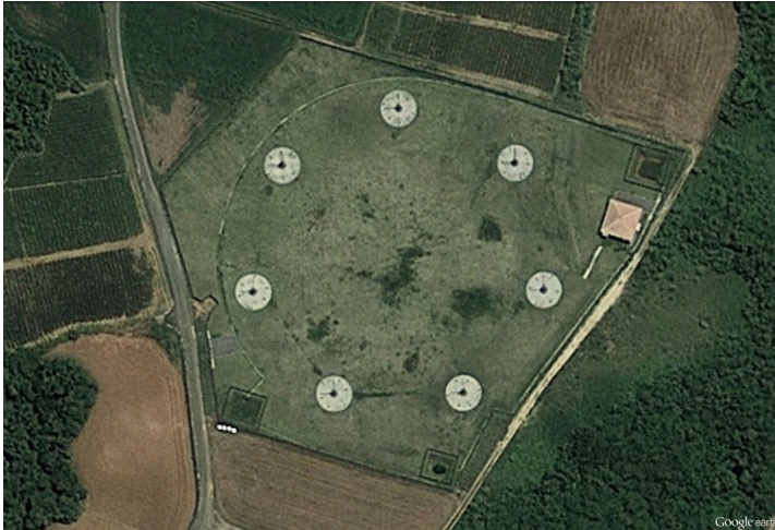
Plate 23. JCG 7-element HF DF station, Ishigaki, 4 July 2010
