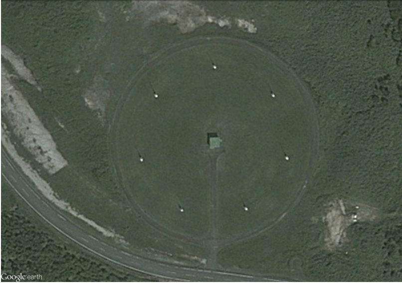
Plate 1. JGSDF Coastal Surveillance Unit 301, Wakkanai, (7-element CDAA for HF/VHF interception and DF), 16 August 2010
