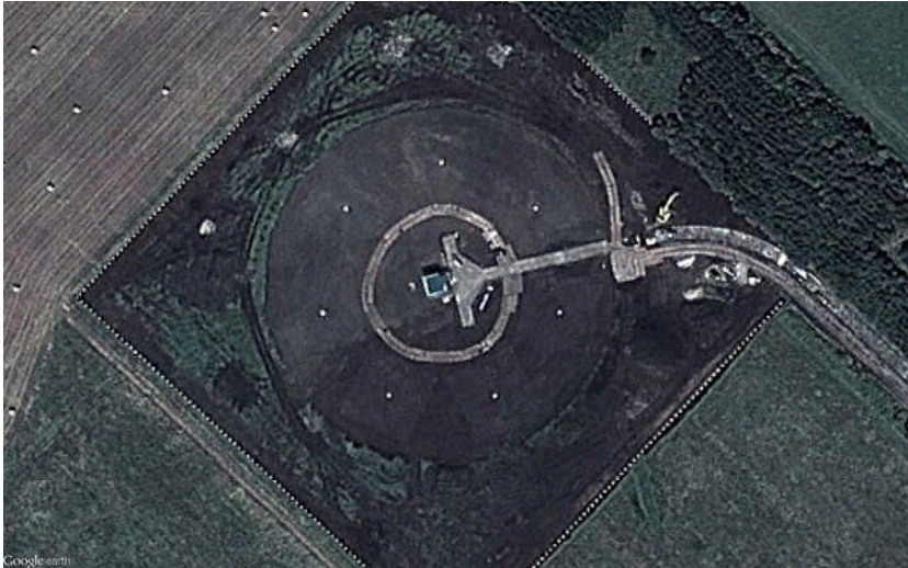
Plate 7. JGSDF Coastal Surveillance Unit 302, Nemuro, (7-element CDAAs for HF/VHF interception and DF), 3 September 2010
