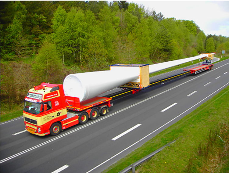
Figure 8.13 Transporting a wind turbine blade (Source: Huson Media).
