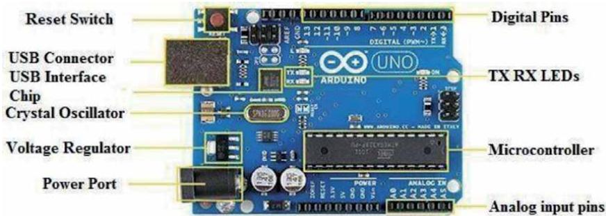
Figure 17. Arduino board.
