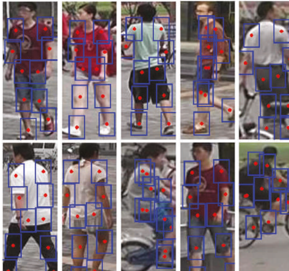
Figure 4. Examples of the segmented ten body parts used in our DJL network.
