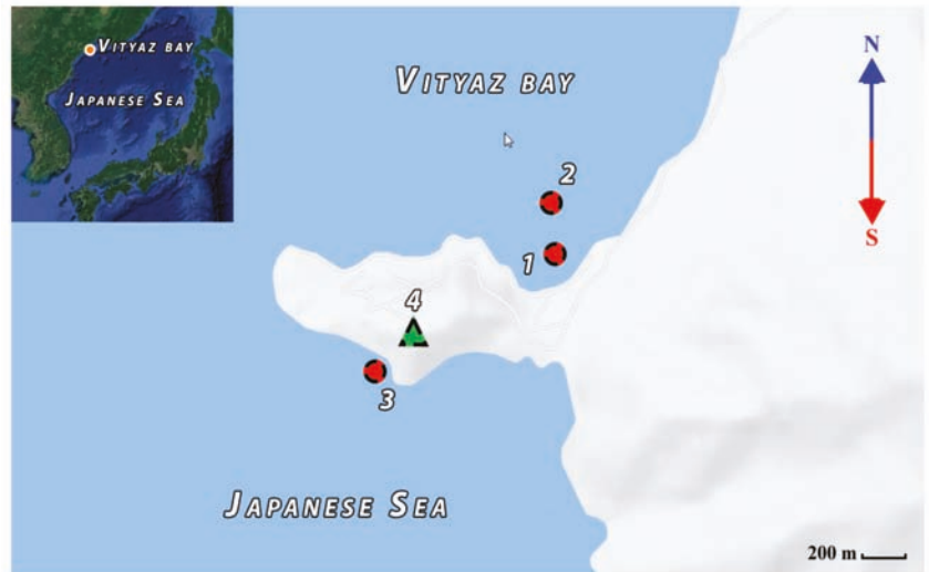
Figure 3. Map scheme of the experimental works. Points 1, 2, and 3 show the positions of laser meters of hydrosphere pressure variations, point 4 shows the position of laser strainmeters.
