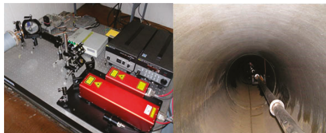
Figure 1. Modernized 52.5 m laser strainmeter. The central interference unit with a frequency-stabilized helium–neon laser, which is stabilized along the iodine lines (frequency stability 10^{-11} , (left)), as well as an underground beam guide (right).
