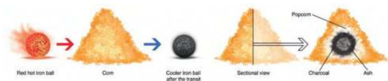
Fig. 8.1 Illustration of passing a hot iron ball through a pile of corn and its effect on the corn
