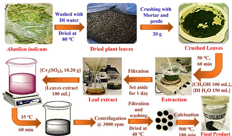
**Figure 10.** The leaf extraction preparation and green synthesis of  $\text{Cr}_2\text{O}_3$  nanoparticles using *Abutilon indicum* (L.) Sweet leaf extracts.
