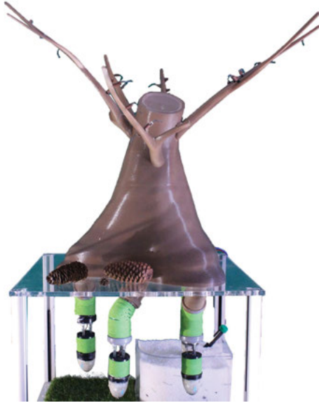
Fig. 1: The plantoid: a bioinspired robot developed at the Italian Institute of Technology, Pisa, Italy, by The Plantoid Project led by Barbara Mazzolai. © Bioinspired Soft Robotics Lab, Italian Institute of Technology, Pisa, Italy.
