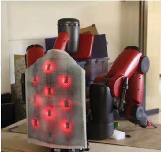
Fig. 2: A soft, amorphous texture-sensitive skin mounted on the back of a Baxter robot. From: [Hughes and Correll 2015, fig. 1]. © 2015 IOP Publishing Ltd.
