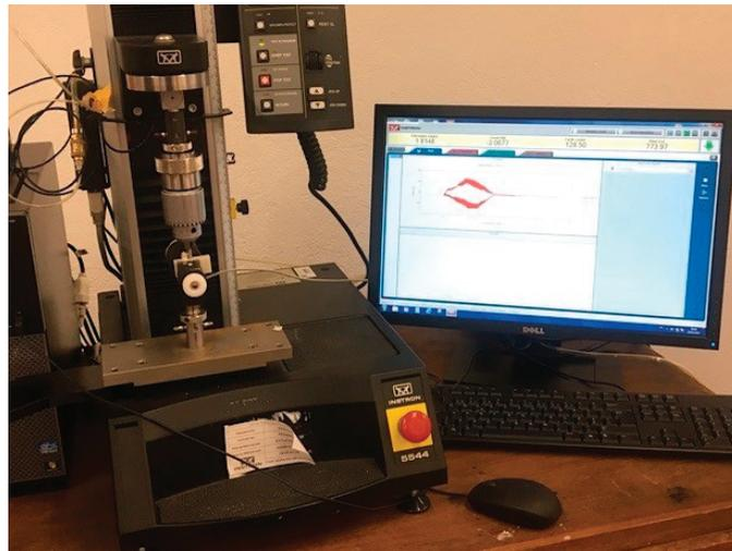
**Figure 10.** Instron 5544 tensile mechanical testing machine.
