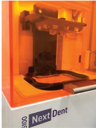
Figure 2. Next Dent 5100 3D printing machine, 3D Systems.
