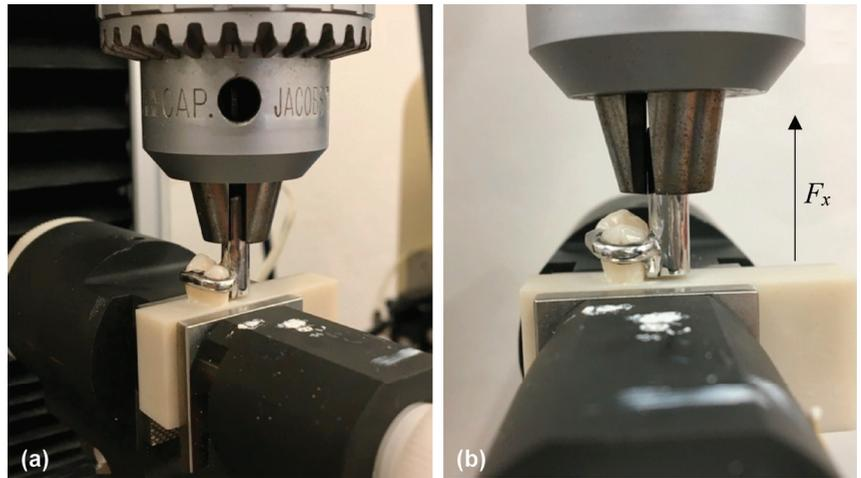
**Figure 11.** Mounting of the test models on the test device, reverse back-action clasp on tooth 1: (a) perspective view, (b) lingual view.
