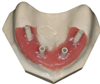
**Figure 1.** Implant level intraoral scan bodies tightened on the reference model.
