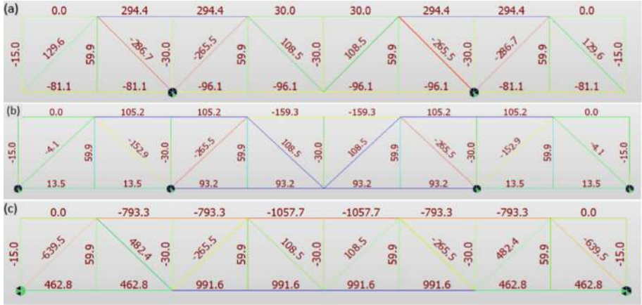
Fig. 1. Internal force of the truss: (a) lifting; (b) installing; (c) completion (kN, negative value represents compression).
