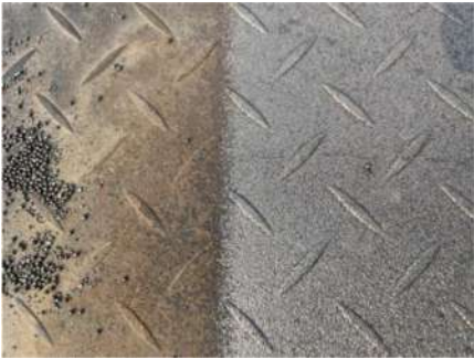
Fig. 5. Shows the steel bridge deck before and after shot blasting on the left
