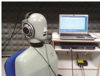
Figure 1. Set-up for measuring the headphones with the Head and Torso Simulator (HATS).
