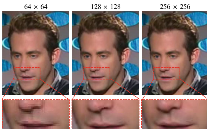
Fig. 4.5 Comparison of DeepFake frames with different sizes of the synthesized faces. Note the improved smoothness of the 256 \times 256 synthesized face, which is used in Celeb-DF. This figure is best viewed in color
