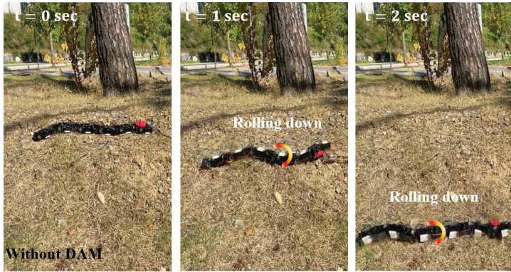
Figure 23. Performance of the descending motion without the DAM on the slope.
