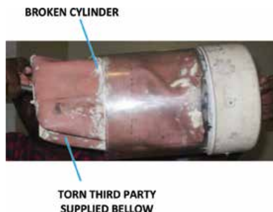
Figure 7. Example of failure during the project.
