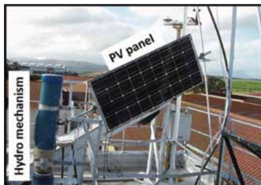
Figure 3. The hydro mechanism driving a sun tracking PV panel (watch online video at: https://www.youtube.com/watch?v=79CKBxt_h-I ).
