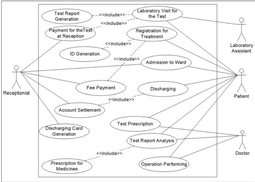
Fig. 12.3 UML use case model of hospital information management process example
