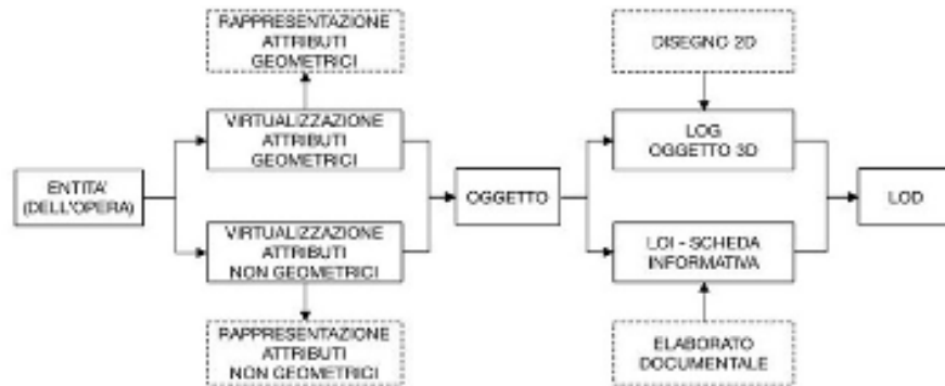
Fig. 6. LOD scheme. UNI 11337-4 (source: UNI 11337-4).
