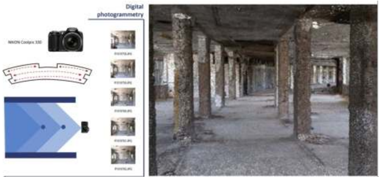
Fig. 7. Point clouds obtained from photogrammetric processes have the advantage of maintaining a high adherence to reality even from a photorealistic point of view (Military hospital in Agnano, survey by M. Siconolfi and S. Monaco).
