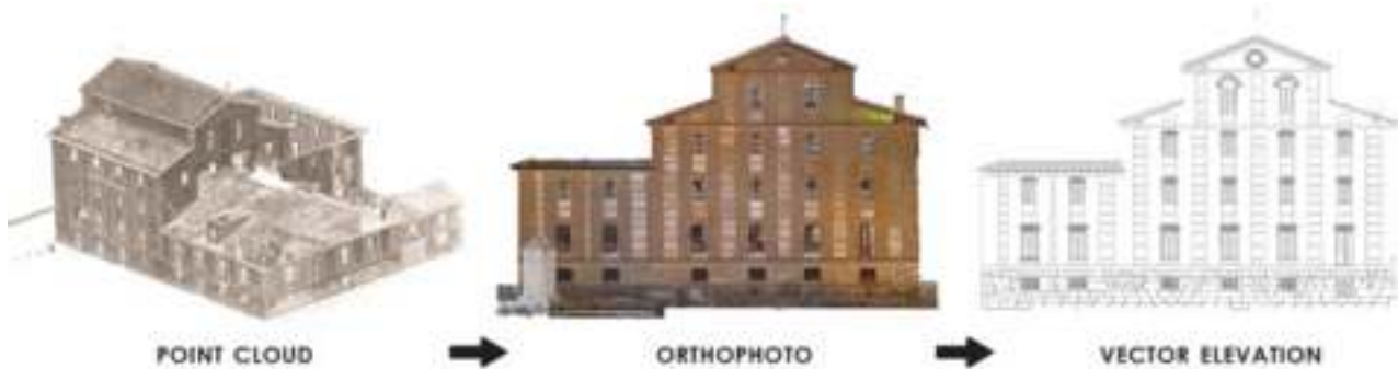
Fig. 4. Process of obtaining detailed documentation from a point cloud model. San Antonio flour factory in Medina de Rioseco (Valladolid) (image: Architectural Photogrammetry Laboratory, Valladolid).
