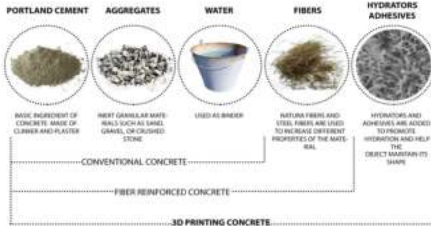
Fig. 8. Reuse concrete recipe mix for 3D printing from construction and demolition activities in the ex-Corradini (image: PROSIT Research Team).
