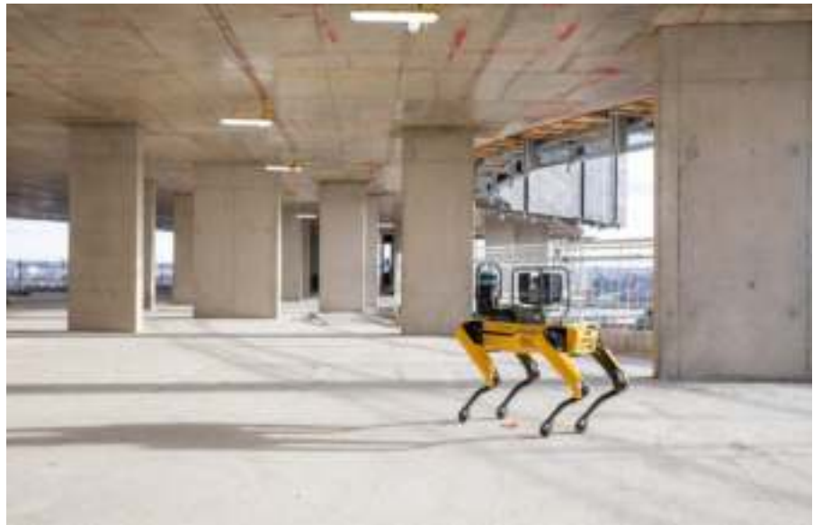
Fig. 4. Use for three-dimensional surveying of Boston Dynamics' "Spot" robot employed by Foster + Partners (source: https://www.dezeen.com/2020/11/13/foster-partners-adopts-spot-the-boston-dynamics-robot-dog/ ).
