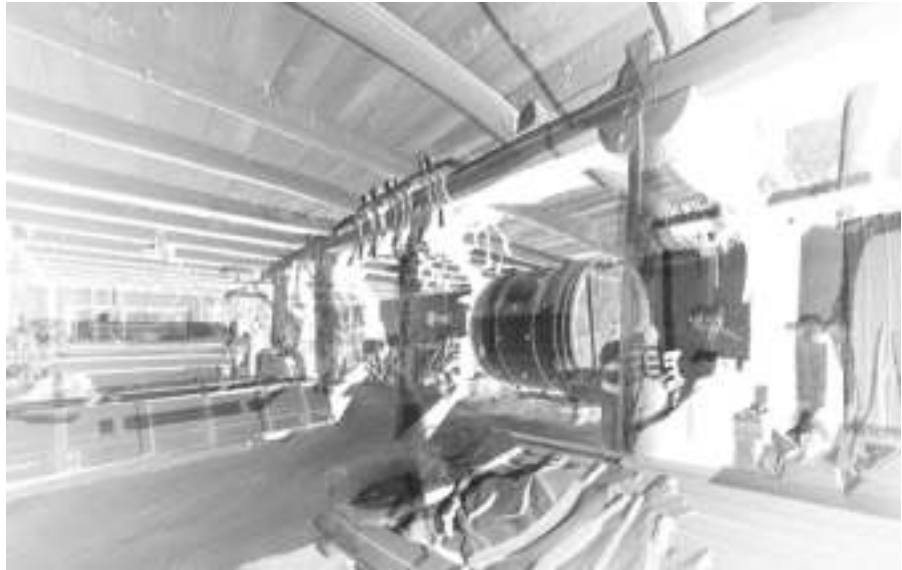
Fig. 2. 3D visualization of a single point cloud obtained using a laser scanner from the Santa María del Páramo tanning factory (León) (image: Architectural Photogrammetry Laboratory, Valladolid).
