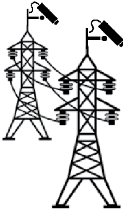
Figure 1. Powerline communication is being deployed for numerous smart grid applications including remote asset monitoring using PLC-based cameras.
