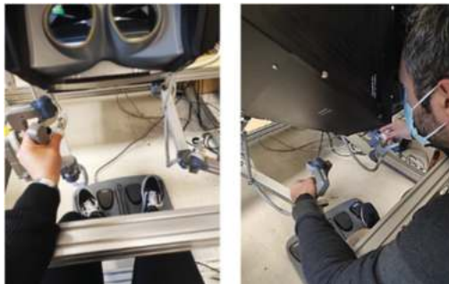
Figure 10. Functionality demonstration. MTM from the dVRK console was used to teleoperate the instrument mounted on the PSM.
