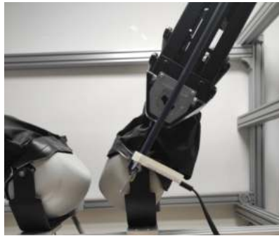
Figure 1. The developed sensing device mounted on the PSM of the dVRK system.
