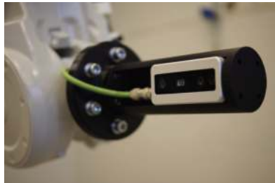
Figure 3. FRAMOS D415e Camera and its bespoke support.
