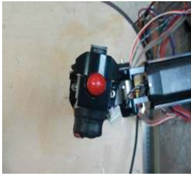
Figure 4. Red marker attached to the end-effector of the robotic arm to calculate the homogeneous matrix.
