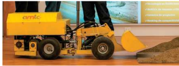
Figure 12. 1:5 scaled LHD built for testing and validation.
