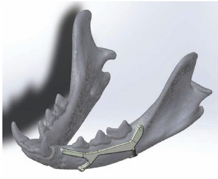
Figure 5. A frontolateral view of the left mandible with the proposed prosthesis. Note the prosthesis thickness is variable depending on the mandibular area in order to fully adapt to its contour. Prosthesis thickness does not exceed 1.2 mm at any point.
