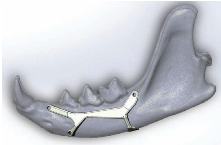
Figure 2. Lateral view of the mandibular prosthesis conceptual model in place, as the upper screws should be fixed where there are no dental roots. This model would be useful to repair body fractures between the third premolar and the first molar.
