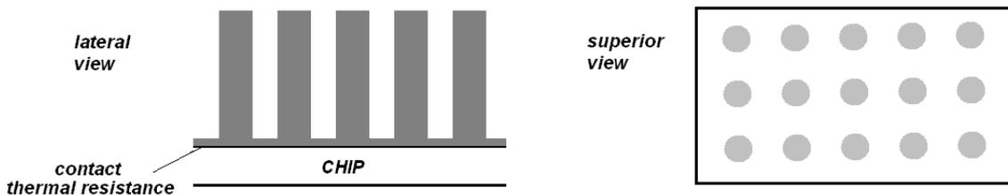
**Figure 1.** Set of cylindrical fins placed on a chip with the aid of a thermal paste (which gives rise to a thermal contact resistance).
