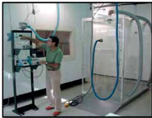
Figure 2. Respirometric chambers for large animal (left) and small animal (right), presented by its designer, professor Norberto Mário Rodriguez.
