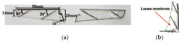
Figure 3. (a) Passive wing rotation mechanism using a loose wing membrane and (b) loosen membrane in moving wing.
