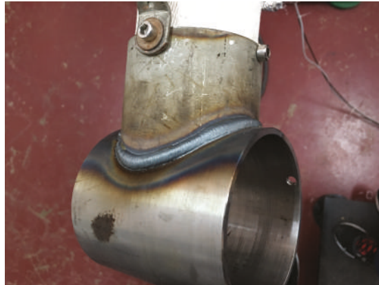
Figure 21. Pipe-connect-pipe arc welding result.
