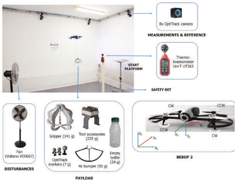
Figure 1. The Bebop 2 quadrotor (and its coordinate system) during one of the initial experiments with the carrying of payload conducted in AeroLab of Poznan University of Technology .
