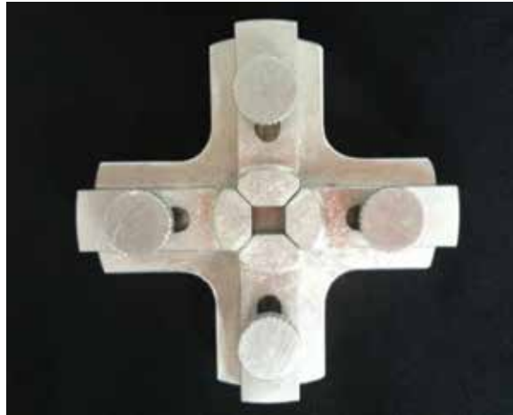
Figure 2. Metallic device where the teeth were fixed for occlusal photographs.
