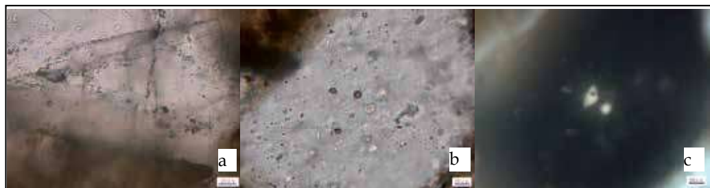
Fig. 3. The two episodes OGIs in Bai 95# oil well, in which, a is the first episode, the depth is 426.8 m; b the second episode, the depth 420.1 m; and c the fluorescence image of b under excited at 365 nm internal light source in the microscope. The scale in a is 20 \mu\text{m} , and in b and c 10 \mu\text{m} .
