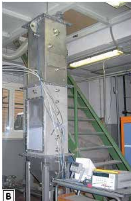
Fig. 7B. 0.35 m side square-based AISI 316 SS unit with tempered glass frontal window.
