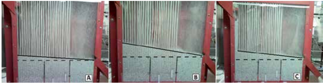
Fig. 13. Continuous operation in the three-module 0.20 m side spouted bed: - - - ideal solids free surface; — actual solids surface at various solids flow rates: a) 2 kg/min, b) 6 kg/min and c) 10 kg/min, as given in the scheme of Fig. 11 B
