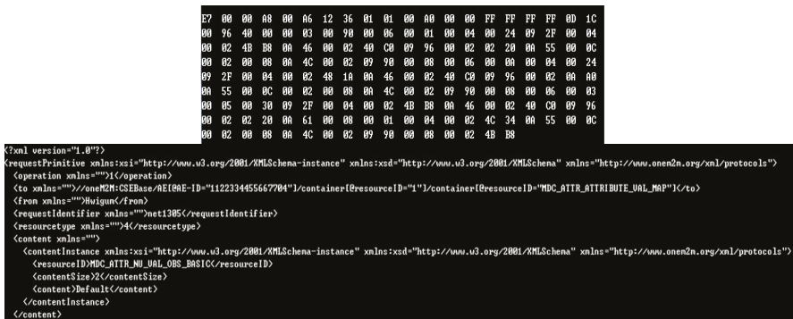
Figure 17. Screen captures of registration (Conversion of an ISO/IEEE 11073 Present (Notice Configuration) Request message into a oneM2M Create primitive Request message).
