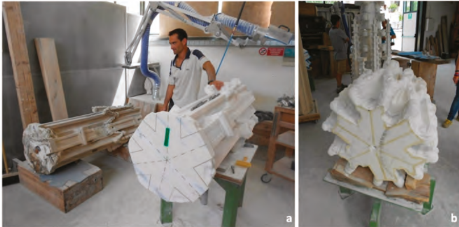
Figure 11. (a) Rough working sketch of the sculpture. (b) Chiselled sculpture to substitute the original one.
