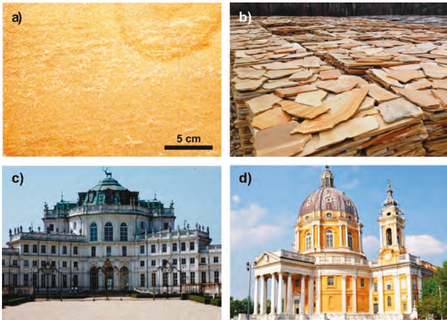
Figure 2. (a) “Golden” quartzite slab; (b) stacked quartzite slabs on the quarry floor; (c) Stupinigi hunting lodge (district of Nichelino in Turin); and (d) Superga basilica (Turin).
