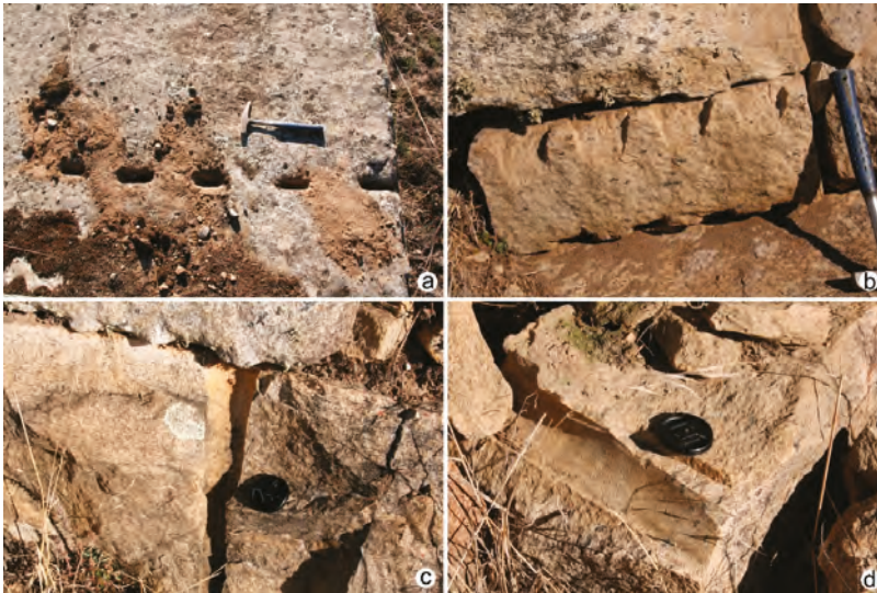
Figure 5. Splitting marks in ancient quarries of Martinamor granite: (a,b) wedge (rectangular) marks and (c,d) triangular-shaped drill holes.
