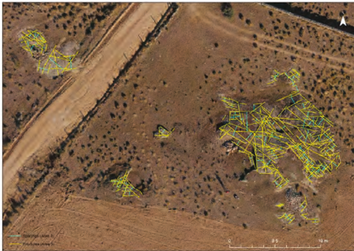
Figure 8. Example of fracturing identification in aerial photomosaic (yellow lines, joints; green lines, joint spacing).
