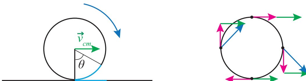
Figure 9.10: Left: illustrating the rolling without slipping condition. The cyan line on the surface has the same length as the cyan-colored arc, and will be the distance traveled by the disk when it has turned through an angle \theta . Right: velocities for four points on the edge of the disk. The pink arrows are the velocities in the center of mass frame. In the Earth reference frame, the velocity of the center of mass, \vec{v}_{cm} , in green, has to be added to each of them. The resultant is shown in blue for two of them.
