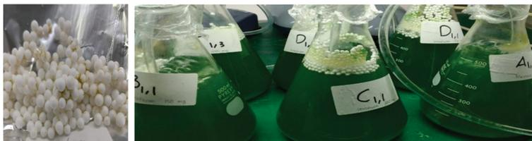
**Figure 1.** Microplastic Styrofoam with a diameter of 2 mm (left) and implementation of Styrofoam in microalgae culture (right).
