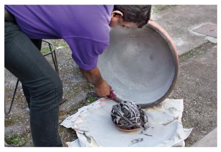
Figure 5: Balendu Prakash opens the Kanduk Yantra (a ball-like apparatus to distill mercury from cinnabar) the next morning; the wrapped-up pre-processed cinnabar had smoldered inside the cotton ball all night. Dehradun, 2013.
