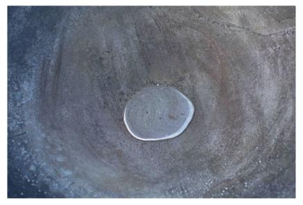
Figure 7: The amount of mercury distilled through the Kanduk Yantra. Dehradun, 2013. This method extracts about 700 grams of mercury from one kilogram of mercury sulfide ore (Prakash 2013, 212).
