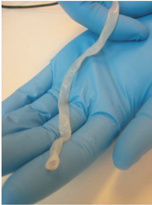
FIGURE 2.1 An artificial blood vessel synthesized by the bacteria G. xylinus .
