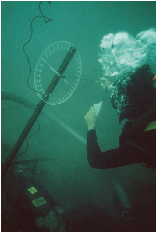
Fig. 3.10 Circular protractor used to record profiles
