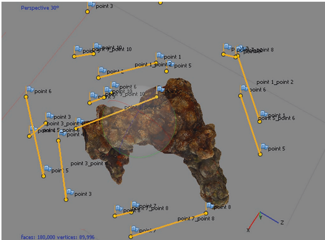
Fig. 4.16 Probable pintle concretion, as recorded (K. Batur)
