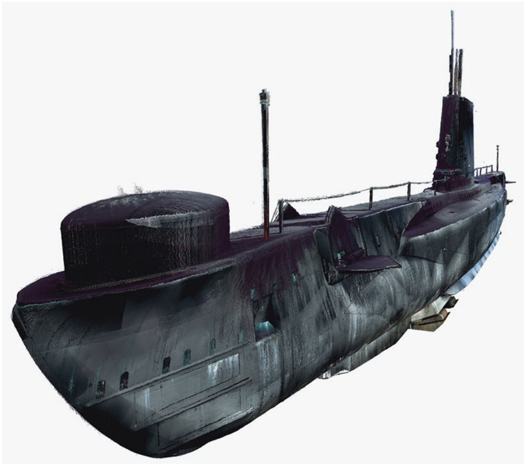
Fig. 7.8 Orthographic representation of the Second World War era submarine HMS Alliance following laser scan survey (Wessex Archaeology Ltd)
