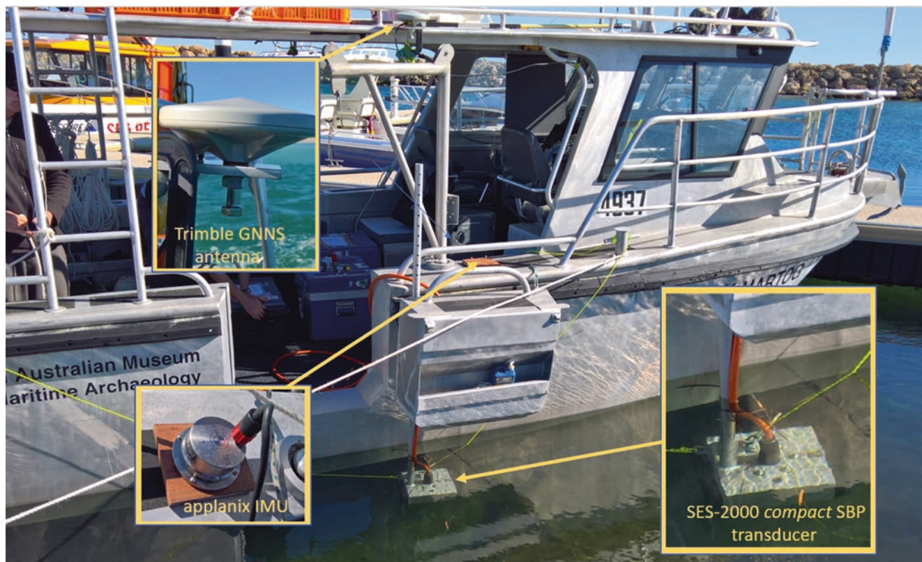
Fig. 10.5 WAM research vessel Dirk Hartog showing mounting locations of SES-2000 compact SBP transducer, Trimble GNSS antenna and applanix IMU sensors
