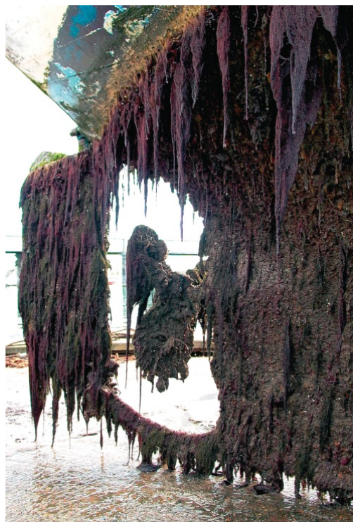
Figure 9.15: Biofouling of a ship's hull with a range of marine organisms.
